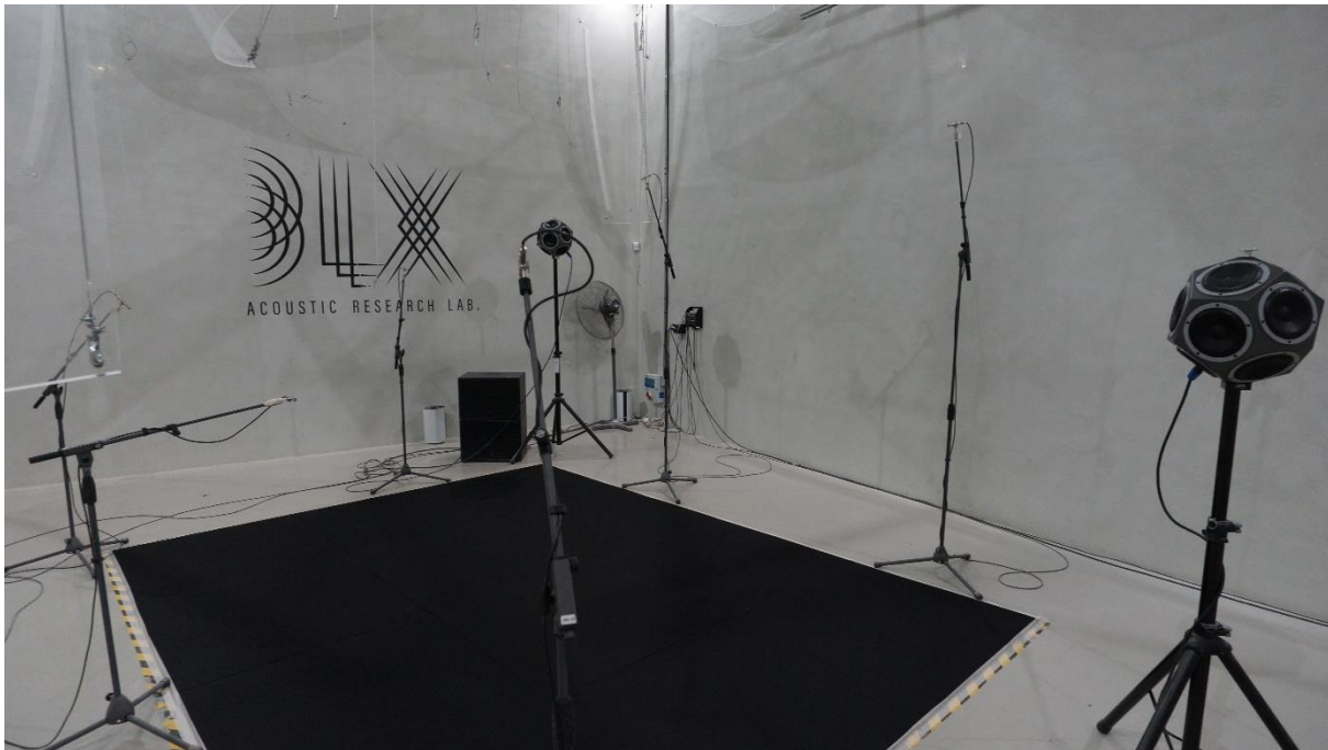
Figure 5.5 Measurement of sound absorption
